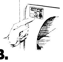
This dryer is equipped for use with NATURAL GAS. You may use manufactured, mixed and L.P. gases with appropriate conversion. No attempt shall be made to convert the appliance from the gas specified on the rating plate for use with a different gas without consulting the serving gas supplier. Conversion must be done by a qualified service technician.
